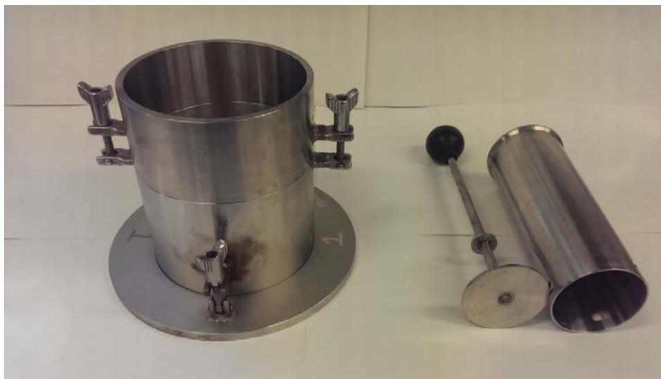
Figure 1 — Example of Proctor/Fagerberg test apparatus, hammer and hammer guide
