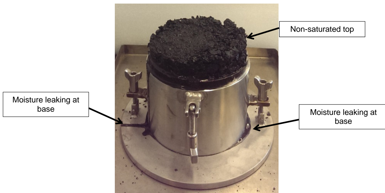
Figure 7 — Test showing water leakage from the base of the cell indicating moisture migration
