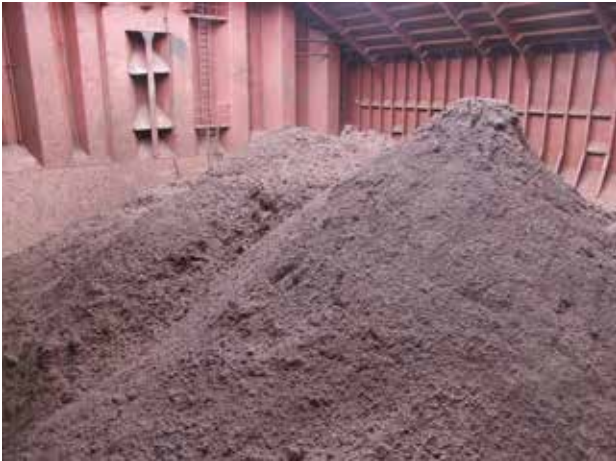
Figure 3: Iron ore fines after loading in the hold of a bulk carrier (Crouch and Aamlid, 2009).
