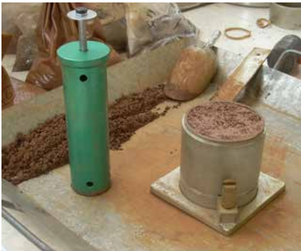
Figure 7: PFT apparatus and compacted sample of iron ore fines.
