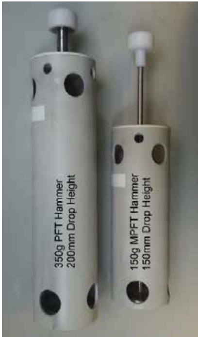
Figure 11: Comparison between the compaction hammers used during the PFT and the MPFT.
