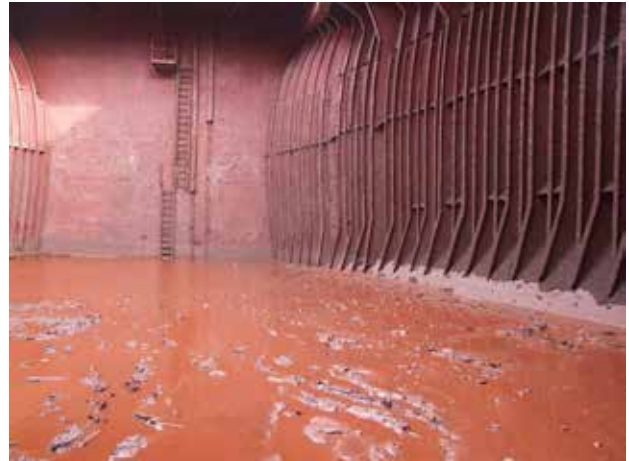
Figure 4: Iron ore fines after transportation in the hold of a bulk carrier (Crouch and Aamlid, 2009).
